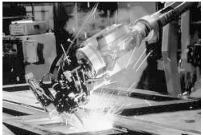
Series BMF 305M/32M-..-W-.. appropriate to extreme applications. Their metal housing makes them resistant to weld splatter build up.
